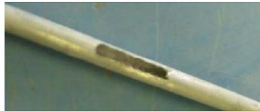
Fig. 9 Slot for grout injection
