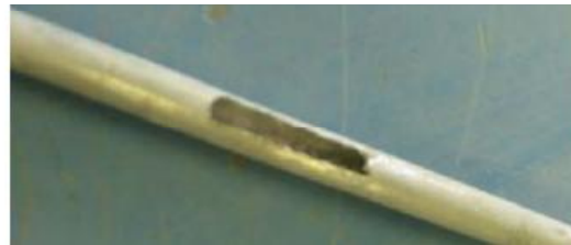
Fig. 9 Slot for grout injection
