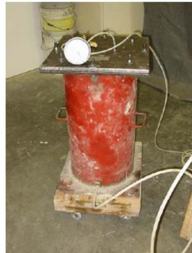
Fig. 5. Pressurized grout cylinder
