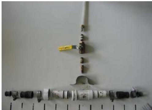
Fig. 10. Grout swivel exploded view
