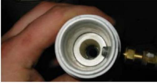
Fig. 12. Grout reservoir
