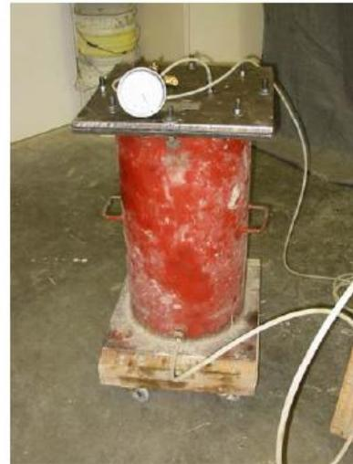
Fig. 5. Pressurized grout cylinder
