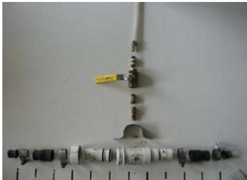
Fig. 10. Grout swivel exploded view
