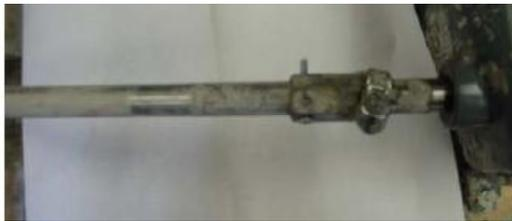
Fig. 8 Pier-motor coupler
