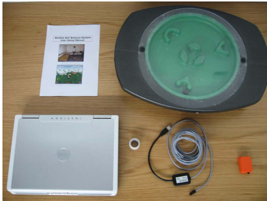
Fig. 1. System components dismantled prior to evaluation session. These include in clockwise from top left corner the instruction manual, wobble board, Xsens MTx motion tracker, Xsens RS-232 cable, Blenderm™ surgical tape, Dell Inspiron laptop.
